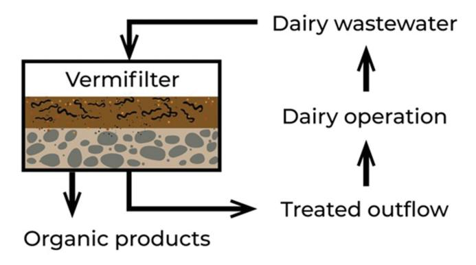
A vermifilter can use composting earthworms to treat dairy wastewater, recycle nutrients, and provide organic products such as fish bait and soil-amending casts. Graphic by Marie Johnston.
