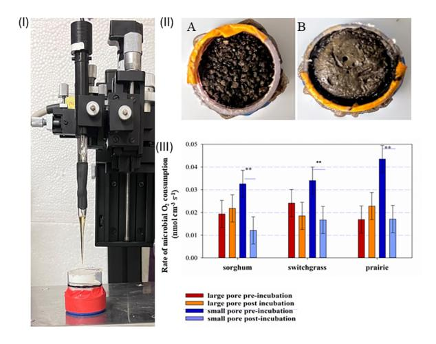
(I) A micro-profiling system with an O2 microsensor; (II) A: large pore soil material, B: small pore soil material; and (III) calculated rates of volumetric O2 by microbes before and after 38 days incubation. Image by Poulamee Chakraborty, GLBRC, Michigan State University.
