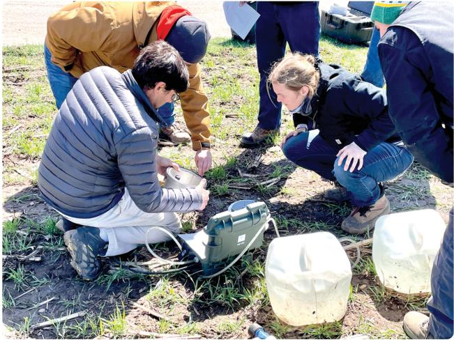
Team conducting training on the SATURO instrument used for measuring water infiltration and permeability, one of the Soil Health Institute's Tier 1 soil health indicators.
