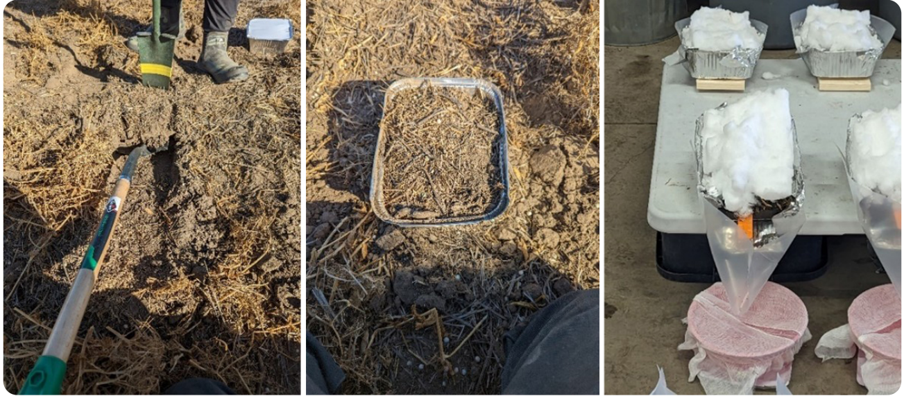
Figure 1. Simulated snowmelt runoff procedure showing intact soil slab removal from plot (left), placement in aluminum tray for storage (middle), and snowmelt simulation (right).
