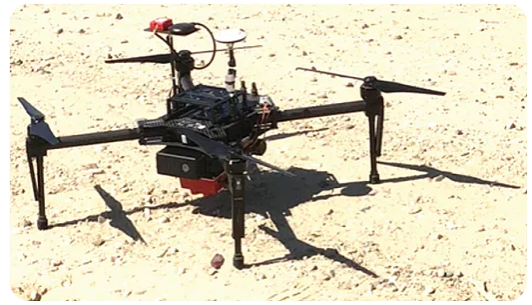
Figure 3. Matrice 100 UAV equipped with the RedEdge-M camera.
