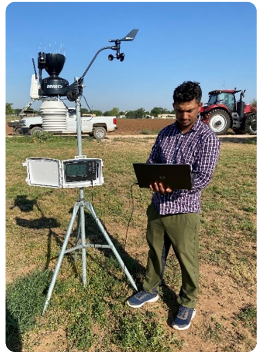
Figure 2. Weather data collection from the Davis Vantage Pro weather station.
