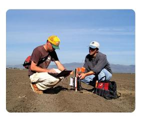
Soil moisture probes track soil salts and nutrients moving through soil profiles with water. Here, research scientists check data being returned from a wireless soil moisture monitoring network, installed in an agricultural field. Photo of courtesy of Forrest S.
