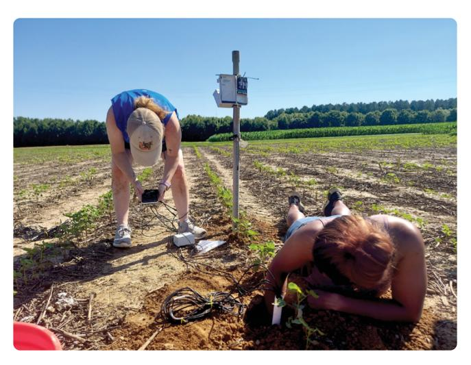
Digital agriculture is emerging as one of the best strategies to de- tect what the crop needs and deliver the right amount of water, nutrients, and other inputs to the crop at the right time and in the right place. Here two lab technicians install a soil water potential sensor in the ground. Photo by Sayantan Sarkar.
