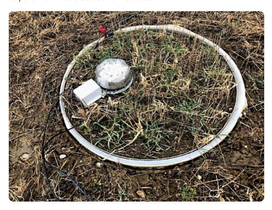
Monitoring for nitrous oxide emissions requires frequent measurements.
