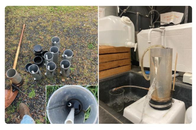
Left: Runoff quantification devices known as UBeTubes are ready to deploy. Inset shows a top-down view. Right: Lab test of the water collected by sampler. Photos by Jacob Maris.
