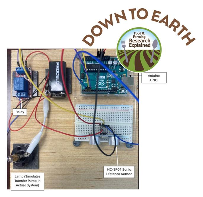
In a Natural Sciences Education study, students used a microcontroller called Arduino UNO to turn on a pair of lights in sequence. This image is the prototype used in developing ChatGPT-generated Arduino programs.
