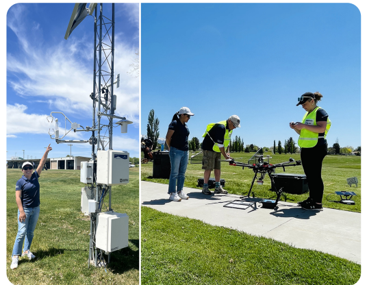
Left: An eddy covariance flux tower. Right: Researchers planning a drone flight at Eagle Lake Golf Course in Roy, UT. Photos by Karem Meza.
