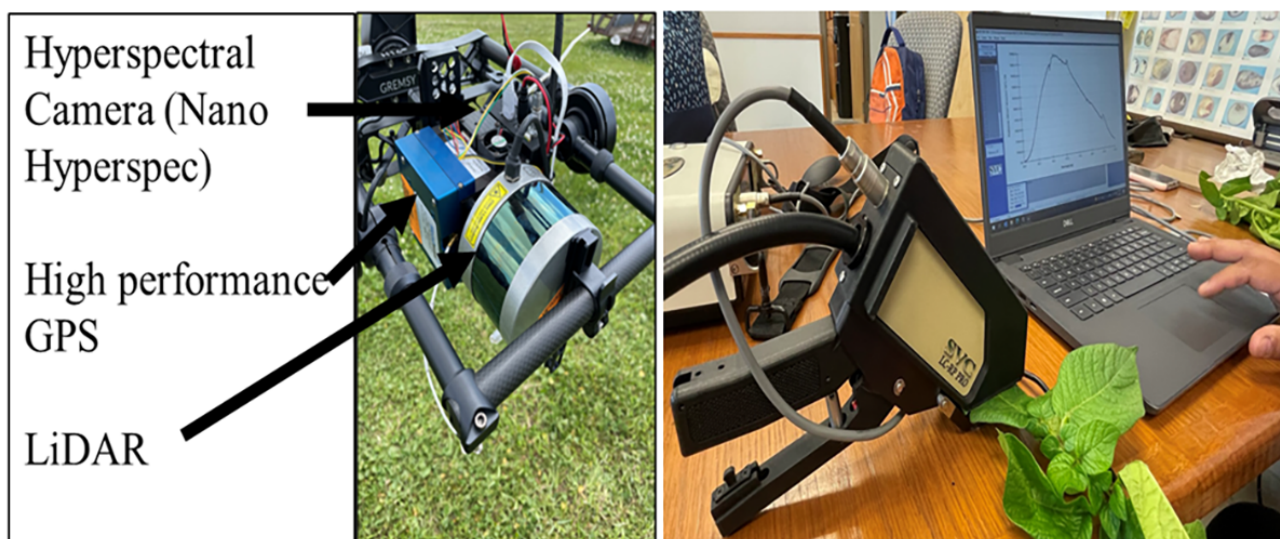
Figure 1. Hyperspectral imaging sensors: mounted on an unmanned aerial vehicle (left) and for leaf scanning (right). Photo by Ayush K. Sharma.
