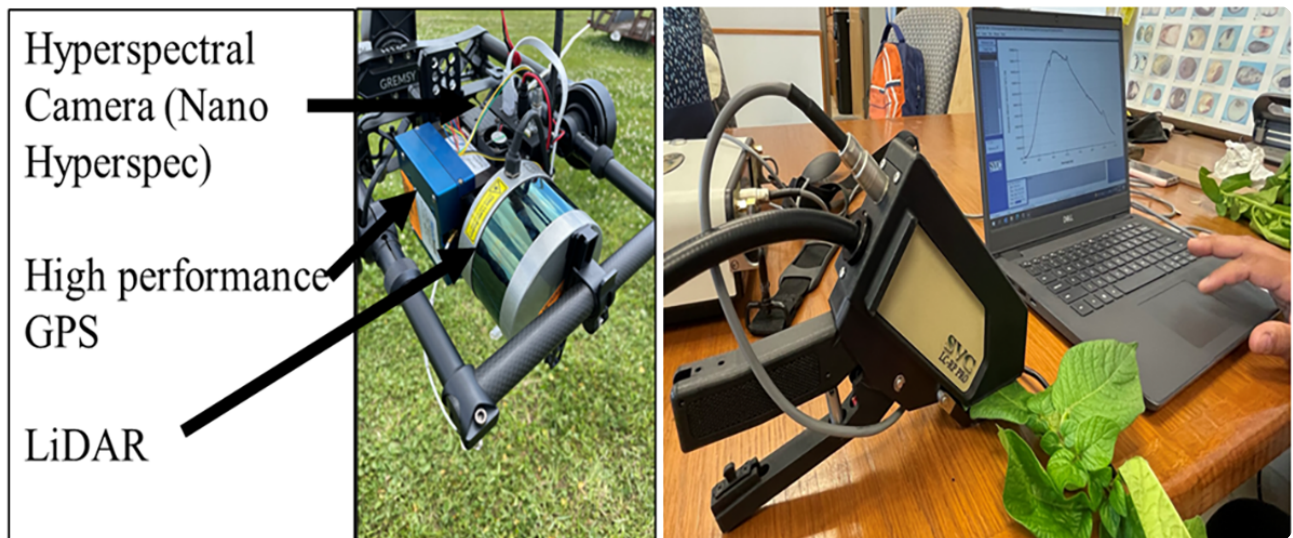
Figure 1. Hyperspectral imaging sensors: mounted on an unmanned aerial vehicle (left) and for leaf scanning (right). Photo by Ayush K. Sharma.
