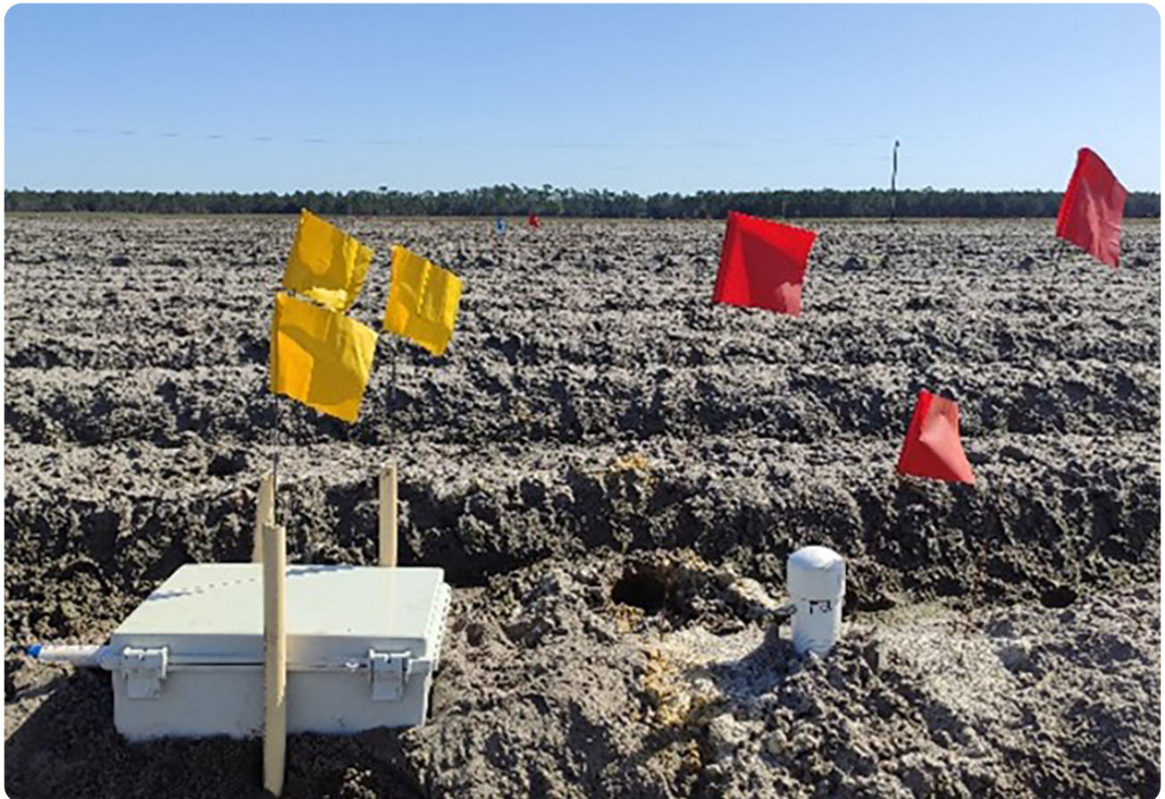
Figure 2. Soil moisture sensor in a potato field, reporting moisture at different depths at 15-minute intervals. Photo by Judyson de Matos Oliveira.
