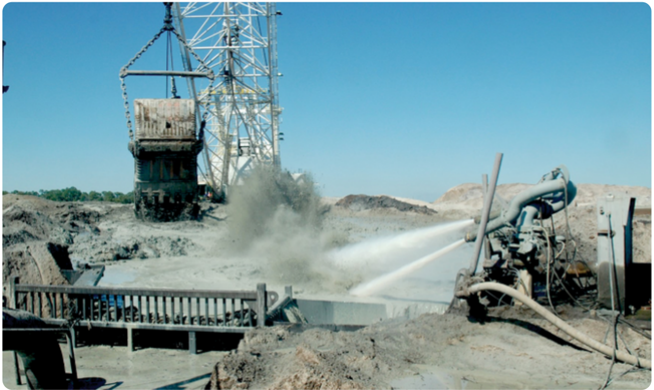
Phosphate ore is converted to a slurry with high-pressure water cannons and pumped to a plant for refining and fertilizer production. Photo courtesy of Alan Blaylock.
