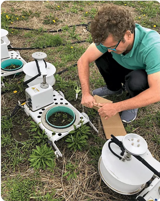
Deepak Joshi, assistant professor of remote sensing and precision agriculture at Arkansas State University, sets up LI-COR long-term chambers in the field for continuous CO 2 and N 2 O emissions measurements. Photo courtesy of Deepak Joshi.
