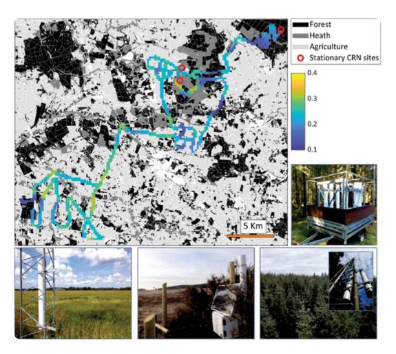
The mean soil moisture (top left) obtained from biweekly surveys con- ducted using mobile cosmic-ray neutron (CRN) detection (top right) in the period December 2018 to May 2019. Bottom: the stationary CRN field sites positioned along the CRN survey route, representing
