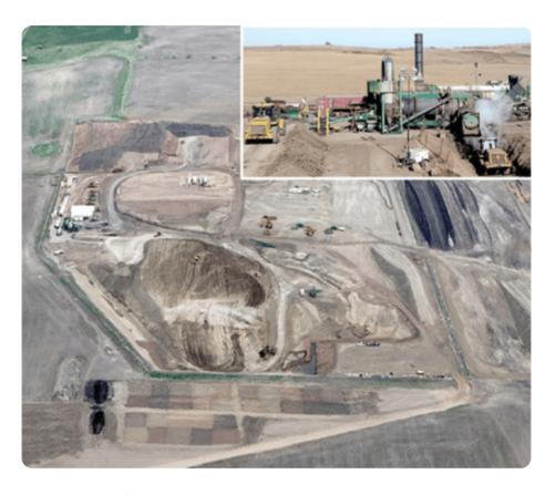
Aerial view of the oil spill remediation site and research plots with inset showing the thermal desorption unit used to treat soils during this project. Photos by Vern Whitten and Peter O'Brien.
