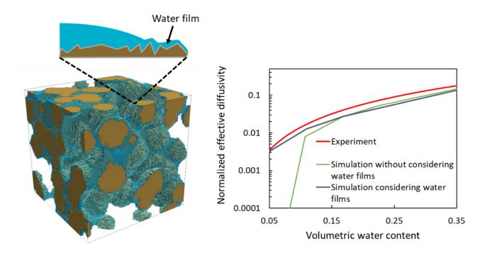
Right: the gas-liquid-solid distribution in the soil microstructure obtained by pore-scale modeling (yellow: solid phase; blue: liquid phase). Left: comparison of the simulation results with and without water films. Image by Yuankai Yang, Forschungszentrum Juelich.
