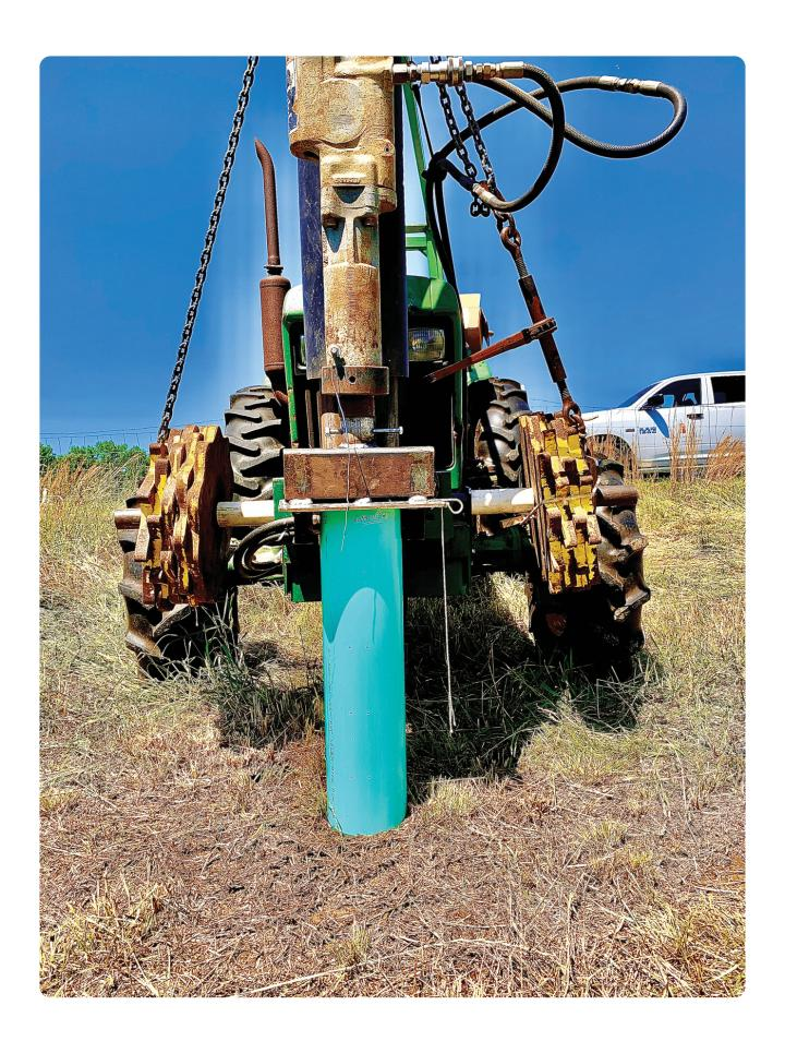
A large intact soil column extracted from a pasture field treated with broiler litter. Photo by Kritika Malhotra, Auburn University.
