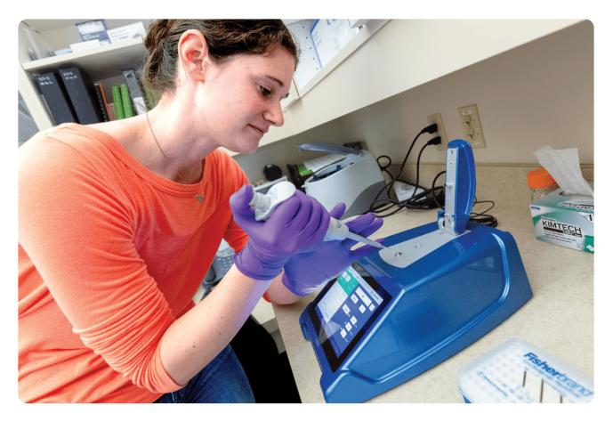
Spectrophotometer for real-time polymerase chain reaction (PCR) testing, which measures DNA amplification to quantify the micro- bial community quantitatively. Photo by NPS/Jacob W. Frank and published under this license: https://creativecommons.org/public-domain/mark/1.0/.
