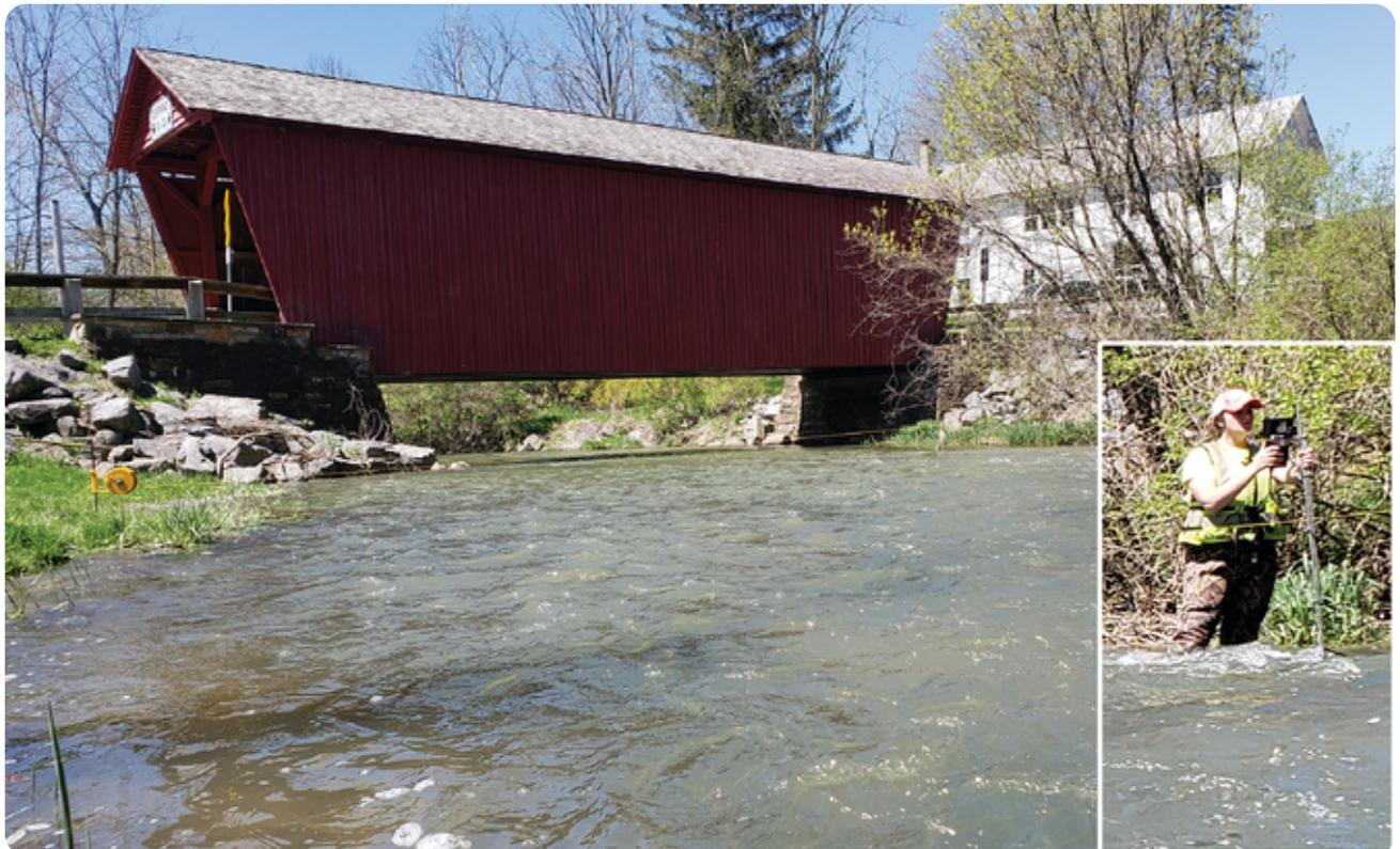
*USGS hydrologist Hilary Dozier measures streamflow above a covered bridge along Fishing Creek in Pennsylvania. Photo by John Clune, USGS.*
