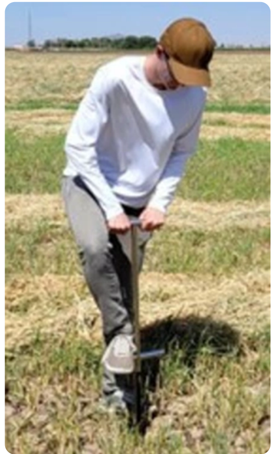
Soil sampling using a soil corer or probe. Image from this publication.
