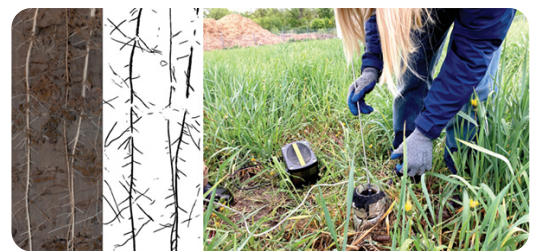
Left panel: Intermediate wheatgrass roots imaged with a minirhizotron (left) and traced with a machine-learning program (right) to study root structure. Image by Alexandra Griffin. Right panel: A researcher images intermediate wheatgrass roots using a minirhizotron. Photo by Emma Link.
