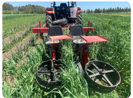
Potatoes were planted directly into the standing rye in late April to early May using a modified no-till transplanter. Photo courtesy of EFAO.
