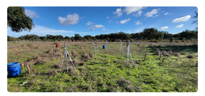
Infiltrometers deployed at an experimental site at Companhia das Lezírias, Portugal. Photo by Pedro Leite.
