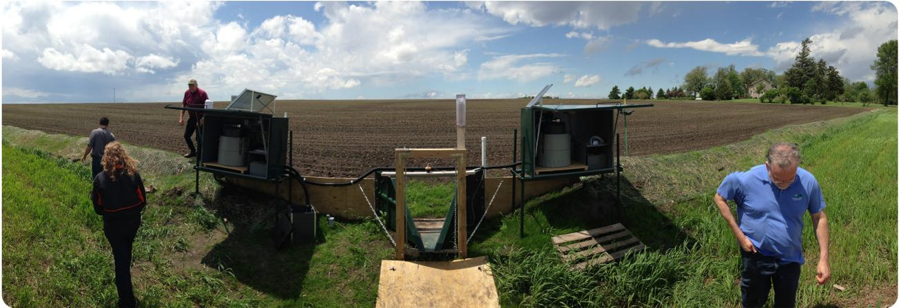
*Fields are monitored using surface water and tile drainage monitoring stations, such as this one in Dodge County, Minnesota. Automated monitoring equipment is shown in the green boxes. Photo by Tim Radatz.*
