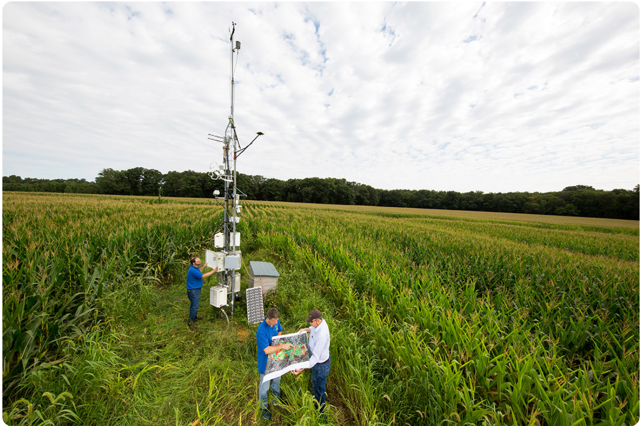
At the Henry A. Wallace Beltsville Research Center, scientists use sensors to monitor carbon dioxide, water vapor, and energy exchanges between the Earth's surface and the atmosphere at a Long-Term Agroecosystem Research (LTAR) field. Photo by Stephen Ausmus, USDA-ARS.
