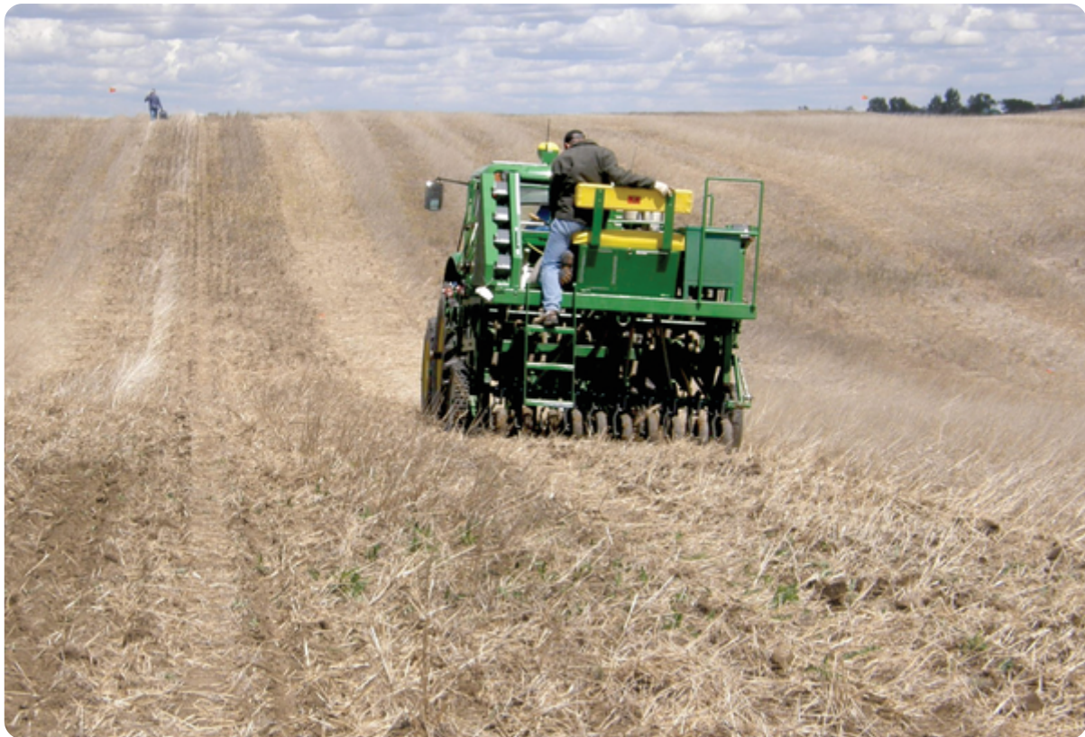
Figure 1. Small-plot seeder establishing strips 7.5 ft in width down the length of the field.
