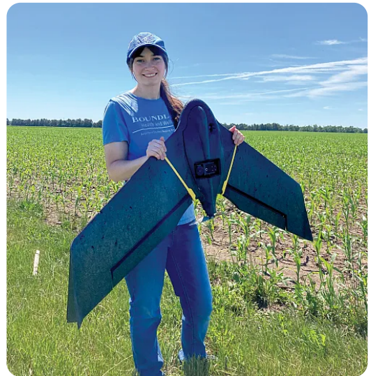
South Dakota State University graduate student Skye Brugler poses with a multispectral drone, which can be used in precision agriculture to capture imaging data
