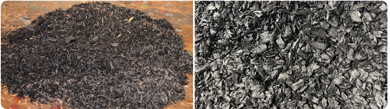
Figure 1. Rice husk (left) and forest wood (right) residues converted into biochar using a small-scale gasifier on a farm in Colombia. Photos by Gustavo Roa and Jaya Nepal.
