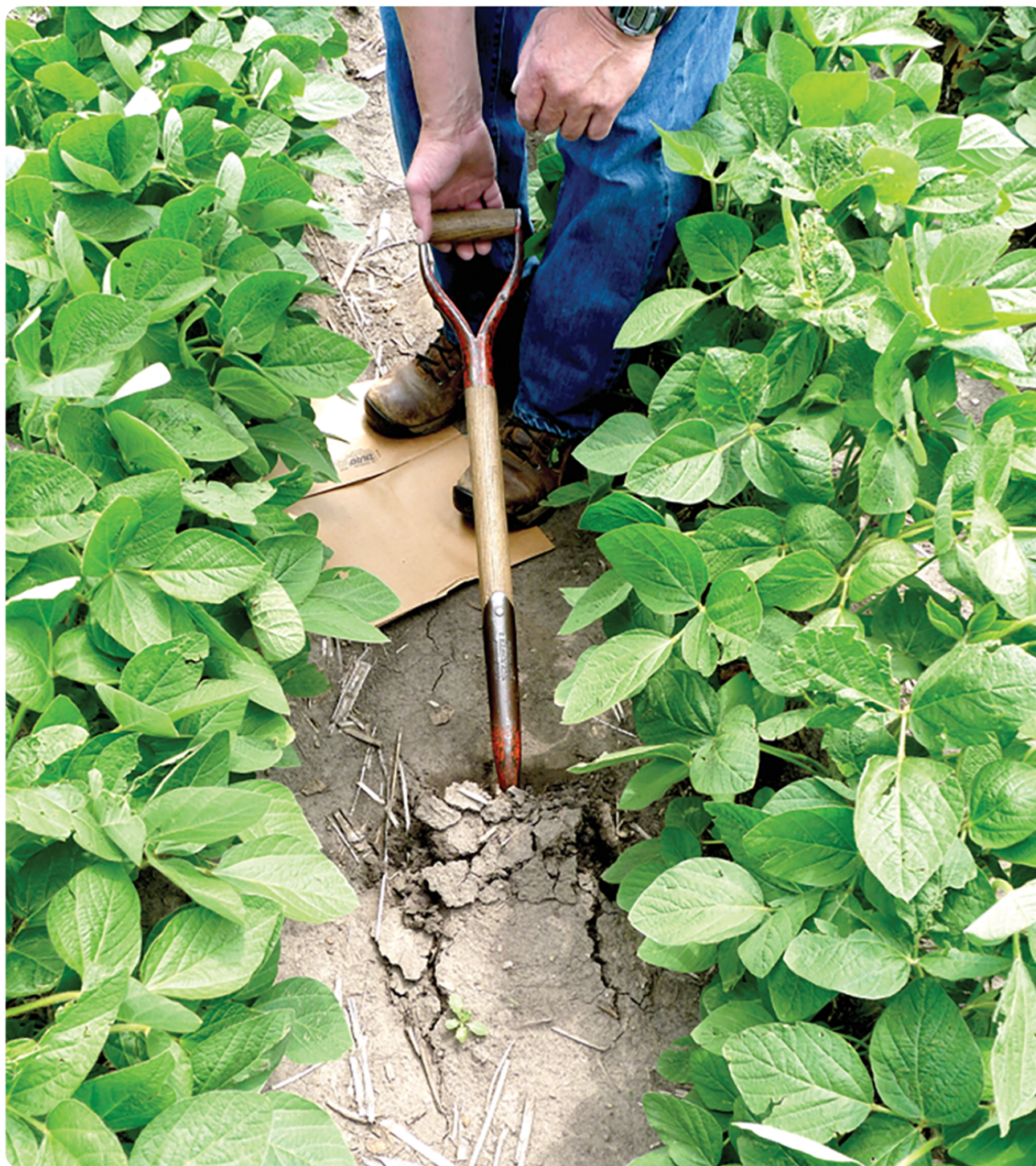
Collecting surface soil for determining wet aggregate stability from soybeans in a field with little surface residue. Photo courtesy of USDA-ARS.
