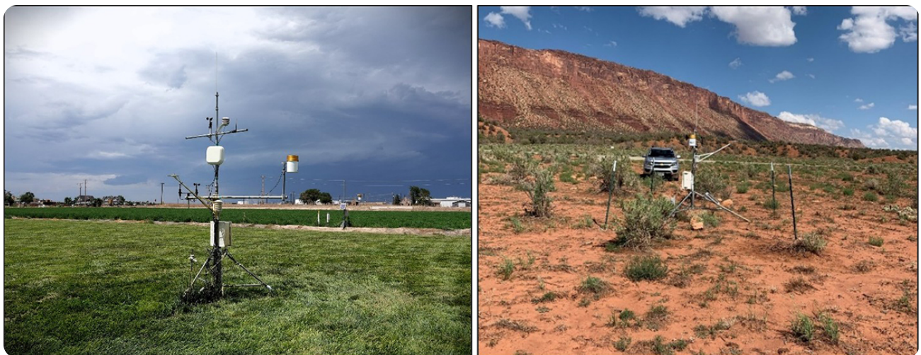
Figure 1. Mesonets and their weather stations can be valuable for many purposes, but stations used for accurate reference evapotranspiration ( ET_{ref} ) estimation should be sited
