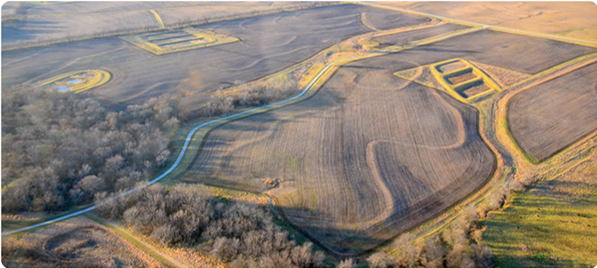
Three constructed wetlands, each made up of three interconnected “cells,” at the Franklin Research and Demonstration Farm. Even one cell filtered significant amounts of nutrients from water coming from adjacent tile-drained farmland. Photo by Tim Lindenbaum.
