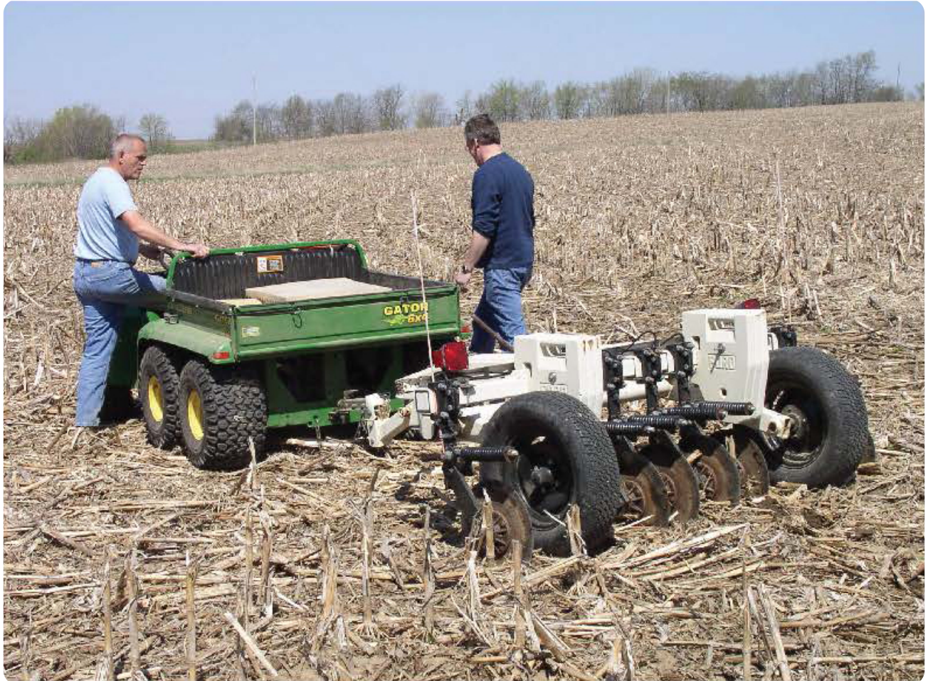
A soil apparent electrical conductivity (ECa) mapping system towed behind a utility vehicle in a field of corn stubble. Photo courtesy of the USDA-NRCS Soil Survey Manual.
