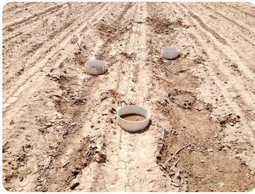
Single-ring infiltrometers being used to determine infiltration rates in a conventionally tilled cotton field near Weinert, TX. Source: Paul B. De Laune.
