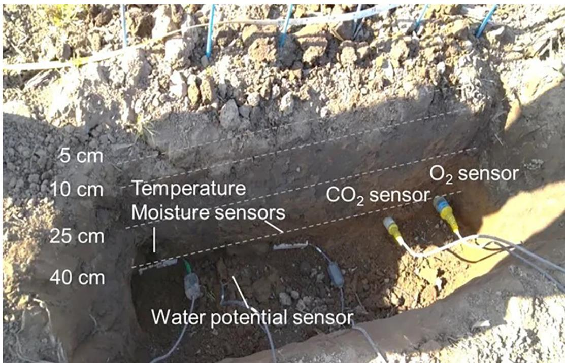
*Field installation of soil sensors used in the study. Monitoring of CO<sub>2</sub>, O<sub>2</sub>, soil moisture, temperature, and water potential was done at multiple depths in a basalt-amended soybean field. Photo courtesy of Yan Zhu.*
