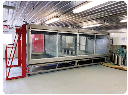
Figure 3, Herbicide spray chamber at the University of Nebraska Pesticide Application Technology (PAT) Laboratory, North Platte, NE.
