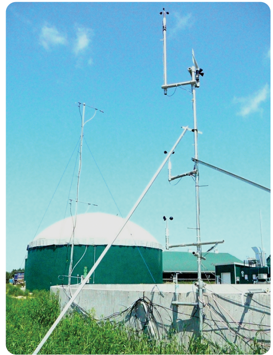
The wind speed measurement tower is shown in the foreground (right), and the air sampling tower is shown to the left with the anaerobic digester as well as part of the dairy barn and generator building in background (from l to r). Source: Claudia Wagner-Riddle.
