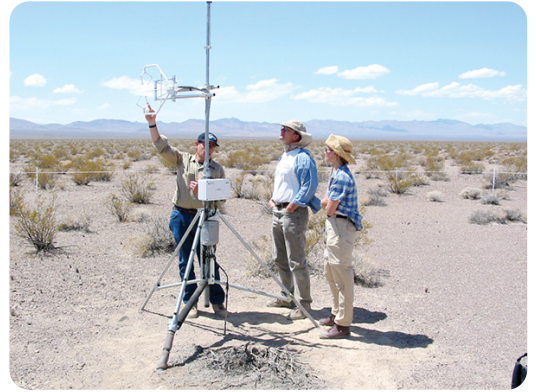
Mike Johnson describing eddy-covariance instruments used to measure evapotranspiration. Photo courtesy of Brian Andraski.
