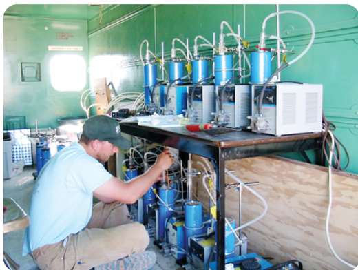
Justin Mayers collecting deep-unsaturated-zone gas samples. Photo courtesy of Brian Andraski.
