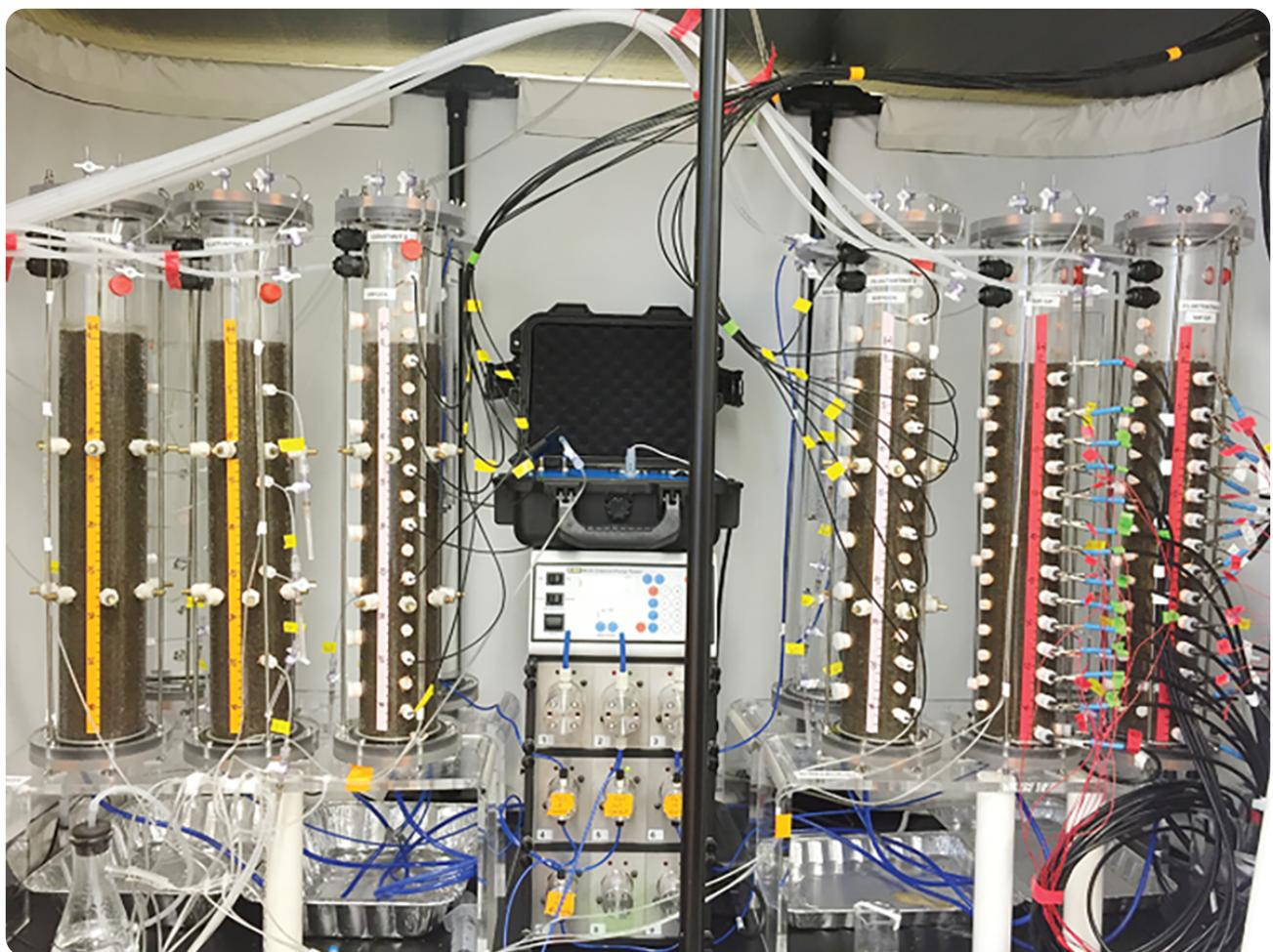
*Automated fluctuating water table soil column experimental setup in which the waterlogged conditions are imposed using a computer-controlled, multi-channel pump connected to a hydrostatic equilibrium reservoir and a water storage reservoir. Photo courtesy of Adrian*
