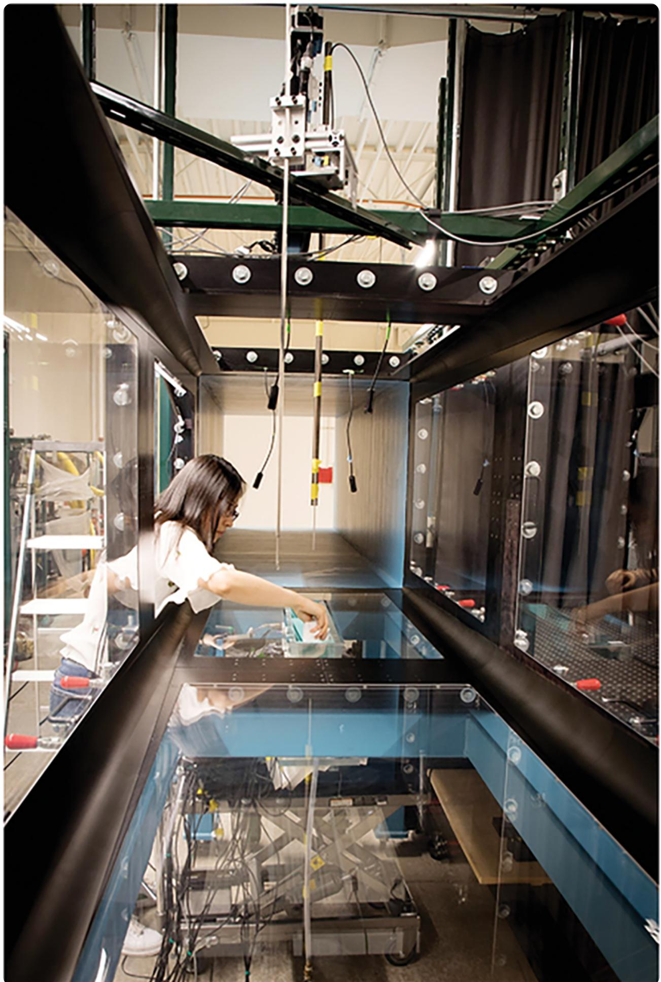
*Graduate student and primary author Bo Gao installs sensors within the soil tank and wind tunnel experimental apparatus. Photo by Kathleen Smits.*
