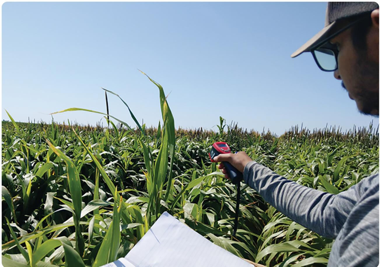
*Bishwoyog Bhattarai, a graduate student in Dr. Sukhbir Singh's lab at Texas Tech University, measuring the canopy temperature using the infrared thermometer. Photo by Sukhbir Singh.*
