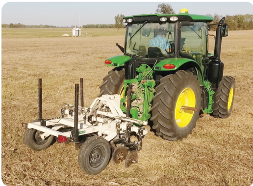
Dr. Ken Sudduth (USDA-ARS) working with a soil apparent electrical conductivity meter (Veris
