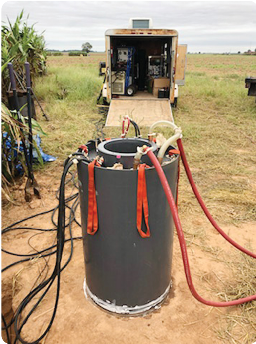
The Texas A&M ROOTS team prepares to deploy its Low-Field MRI system to non-destructively image roots. Photo courtesy of Cody Bagnall, Texas A&M University.
