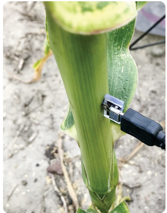
A microneedle-based nitrate sensor capable of real-time, in planta measurements in the field. Photo courtesy of Liang Dong, Iowa State University.
