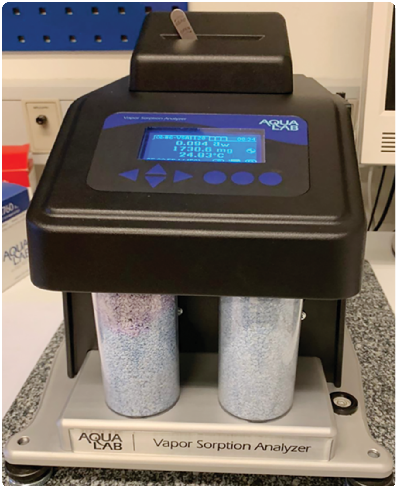
The vapor sorption analyzer provides sorption isotherm measurements by automatically wetting and drying the sample while recording the change in the sample mass. Photo by
