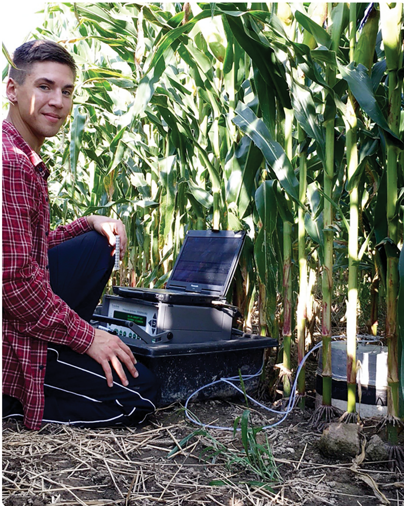
Kyle M. Dittmer capturing greenhouse gas fluxes with a photoacoustic multi-gas analyzer from a corn silage system located in Alburgh, VT. Photo courtesy of Kyle Dittmer.
