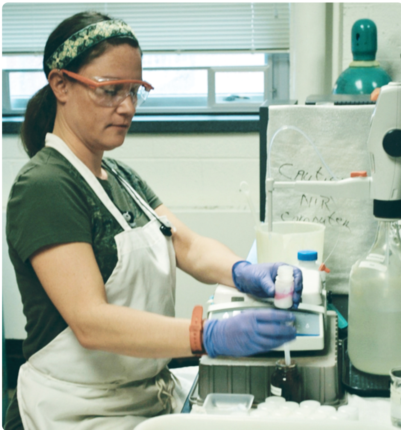
Lab technician, Erin Silva, prepares a sample for titration with hydrochloric acid to determine the amount of CO 2 released by soil during incubation as part of soil-test biological activity to predict soil nitrogen mineralization. Photo by Alan Franzluebbers, USDA-ARS.
