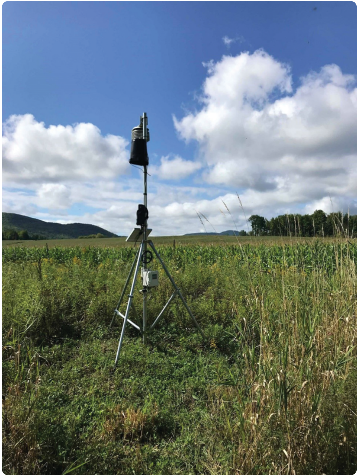
The weather station at my research site in northern New York during the growing season. The station measures air temperature, pressure, relative humidity, and rainfall every hour throughout the year. This monitoring device is crucial for characterizing the
