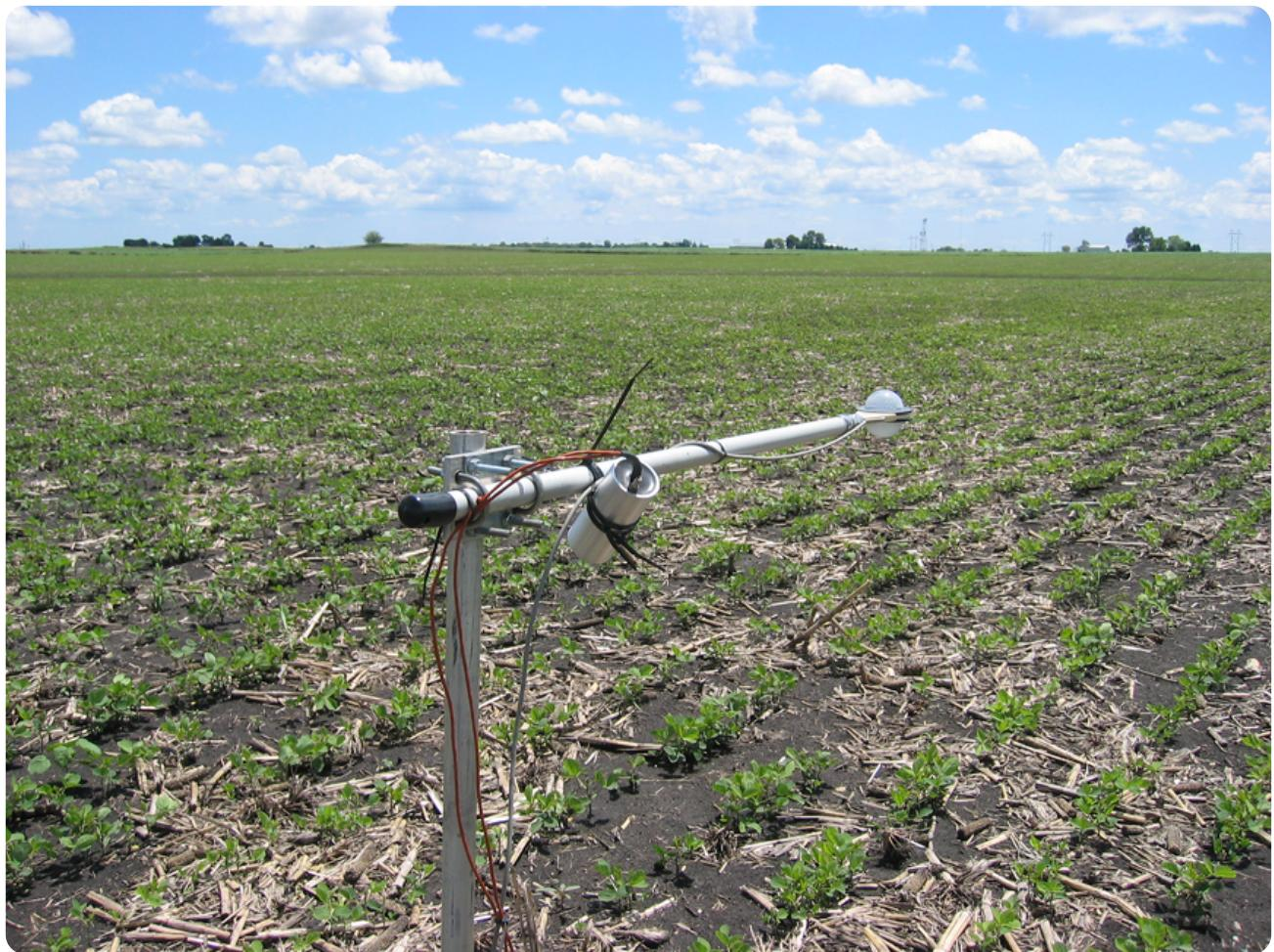
*Infrared radiometer monitoring surface temperatures in an Iowa soybean field in mid-June.
