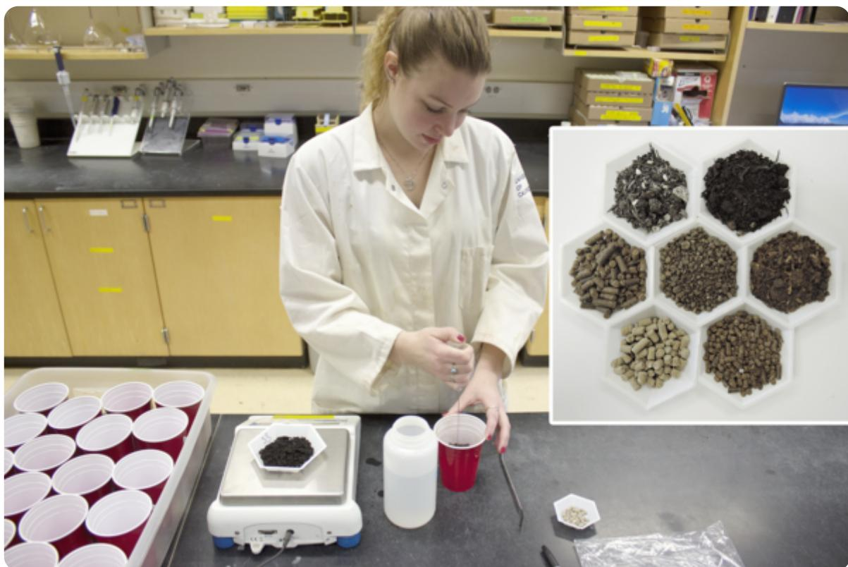
*Amendments were mixed with soil, adjusted to optimum moisture, and incubated in plastic cups for 1, 3, 6, and 12 weeks.*
